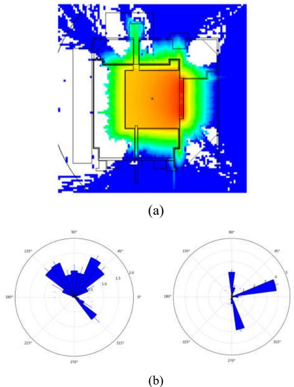
Fig. 4. Vertical profile cross section of (a) the GR 440 with a dose rate scale showing the lowest dose (blue) below 50  $\mu$ Sv/hr and (b) the external radiation fields in units of mrem/hr (as shown on the diagonal axis) from twenty-four measurement points (left) around the circumference of the system and (right) from the left side and over the top to the right side of the system with respect to the orientation shown in (a).
