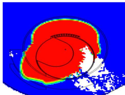
Fig. 5. Horizontal profile cross section of the GR 440 with a dose rate scale showing the lowest dose (blue) below 50  $\mu$ Sv/hr and highest dose (red) as greater than 0.5 mSv/hr at the point of greatest penetration of the transient dose to visualize the gradient at the edge of the lead door when changing between irradiation and loading modes of operation.
