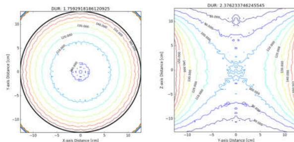
Fig. 2. Overall GR 440 irradiation field parameters including a dose uniformity ratio of 2.37 for the radius versus height isodose profile (right) and 1.76 for the horizontal radial plot at the midplane of the chamber height (left) with a centerline dose rate of 127.0 Gy/min. Field lines in the isodose profiles are labeled by percent with respect to the centerline dose rate.
